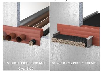
The FF260 Fire Protection Block is made of a rapidly expanding intumescent foam and the **ideal fire barrier for cable, pipe or mixed penetrations, as well as blank openings** in solid floor or ceiling systems. The flexible and lightweight material is suitable for retrofitting installation, as well as new construction and can be used for openings up to 384 in<sup>2</sup> with a maximum dimension of 32".
