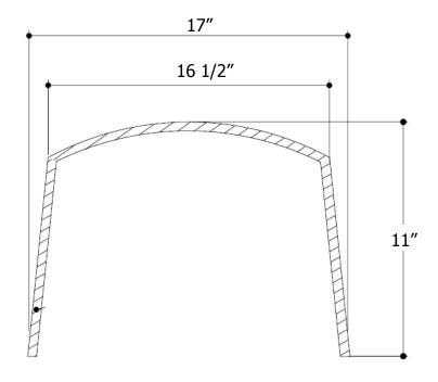
FLEXIBLE TO FIT 16" ON CENTER JOISTS
