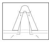
When installing from above and fixing wire is not required, the FF130R can alternatively be bonded to the ceiling with a bead of silicone sealant.
