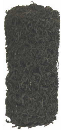
Intumescent material expands at 375° F up to 25x its original thickness.
