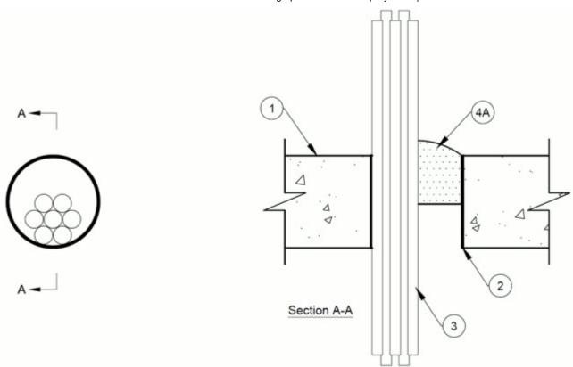
1. **Floor or Wall Assembly** — Min 4-1/2 in. (114 mm) thick reinforced lightweight or normal weight (100-150 pcf or 1600 - 2400 kg/m<sup>3</sup>) concrete. Wall may also be constructed of any UL Classified **Concrete Blocks\*.** Max diameter of opening is nom 5 in. (127 mm).
